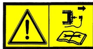
Remove the spark plug wire before maintenance
