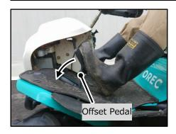
Pushing offset pedal by left foot enables to manually open/close the offset deck. Offset deck is open when foot leaves the pedal.
