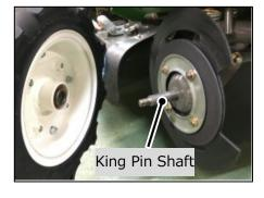
Clean inside of tire wheel. Before to assemble this part, do not forget to grease up and lubricate the king pin shaft. .
