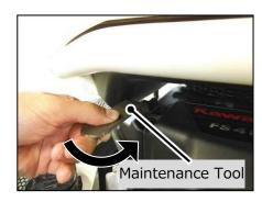
1) Use the maintenance tool to remove air cleaner cover.
