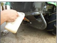
Place the drain plug in original position. Remove the transmission plug and then put transmission oil.
